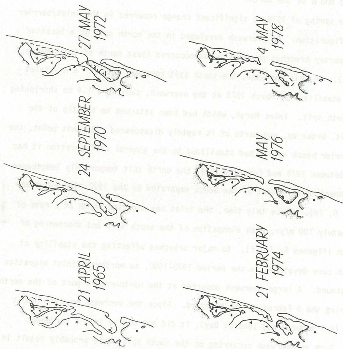
Figure 7. Tracings of vertical aerial photographs of Nauset Inlet between 1965 and 1978.
