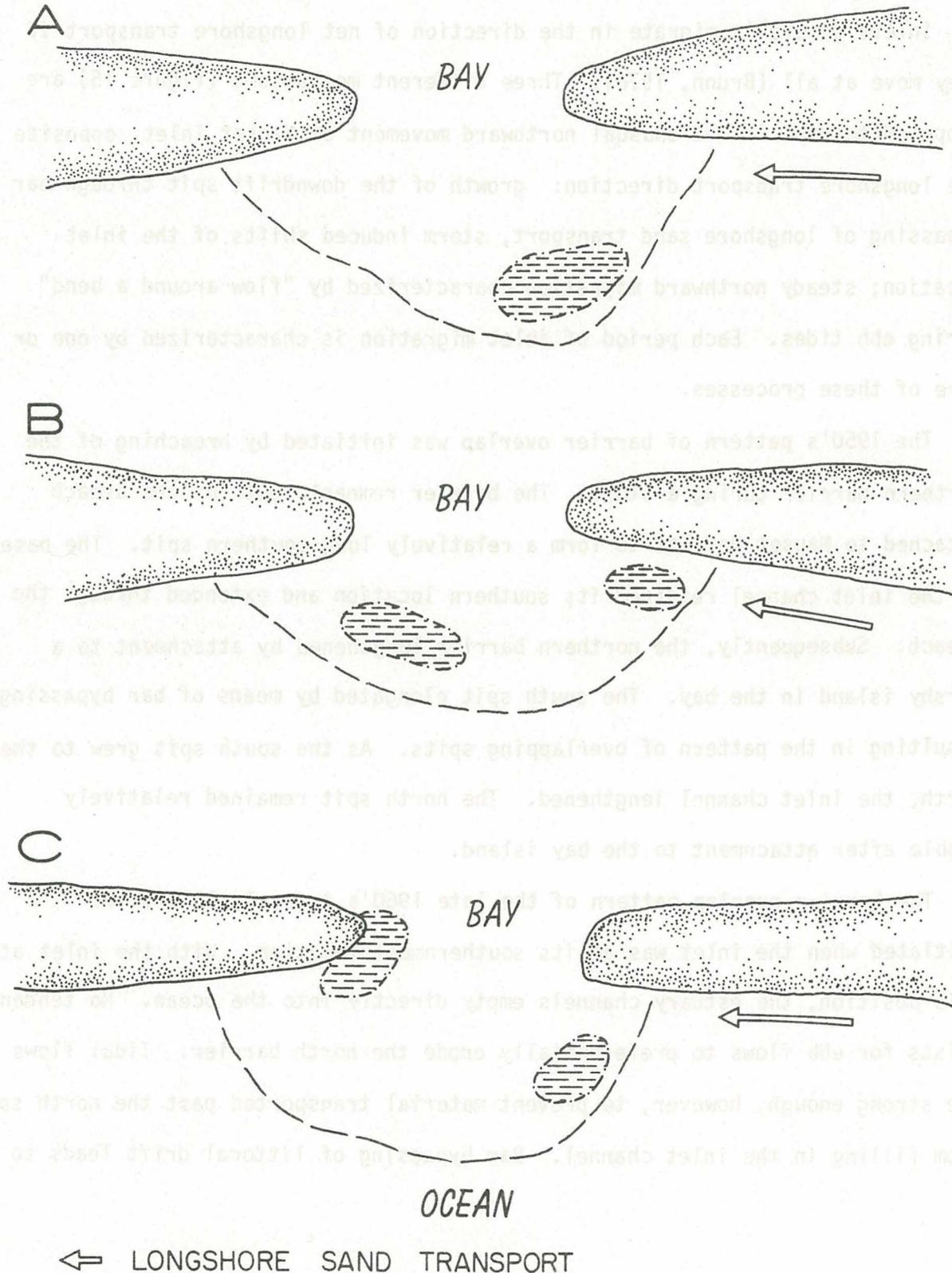
Figure 15. Three modes of updrift inlet migration responding to different combinations of waves, tides and storms. All three modes have been observed at Nauset Inlet, Cape Cod, Massachusetts.
