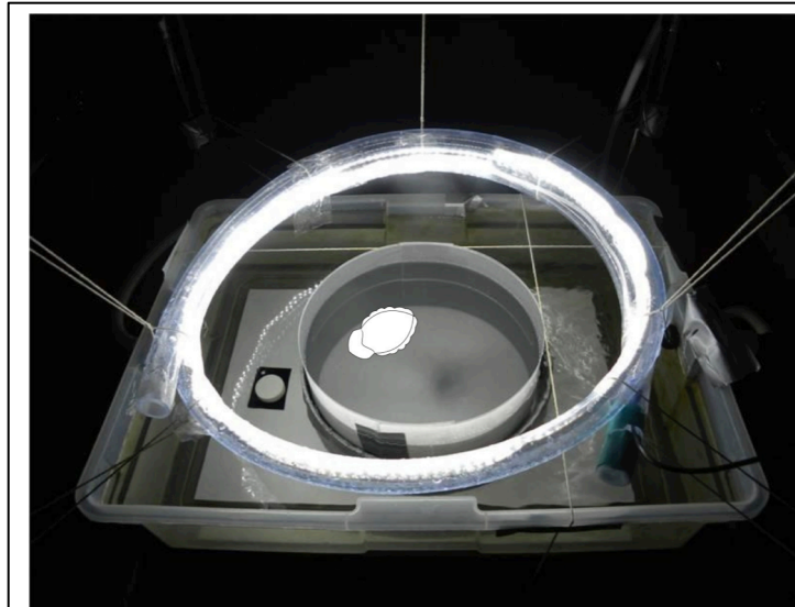
Figure 5.2 Experimental and photographic setup. The circular cuttlefish arena was placed in a rectangular tank supplied with seawater circulation. The setup was illuminated with a ring-shaped LED light, above which the camera was mounted looking down (not shown in photo). Black and white calibration targets were placed inside the rectangular tank (shown here on the left), out of the field of view of the animal in the circular arena and remained in the same location throughout the duration of the study.
