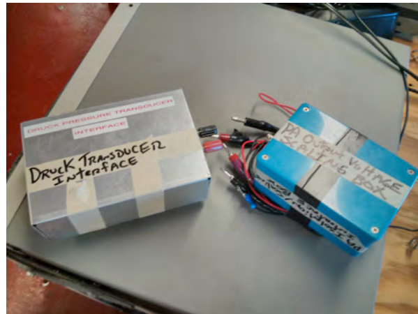
Figure 19. Druck Pressure Transducer Interface Box & PA Voltage Isolation/Scaling Box
