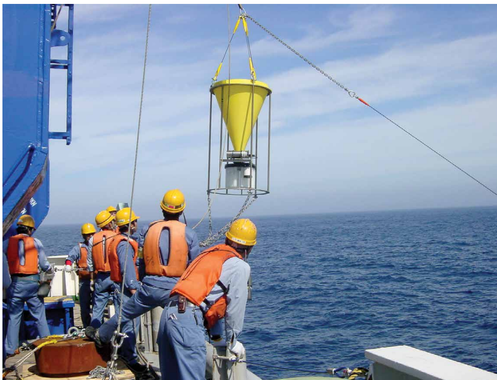
Figure 4. Time-series sediment trap being deployed off Japan on JAMSTEC ship R/V Mirai . Photo credit: M. Honda
