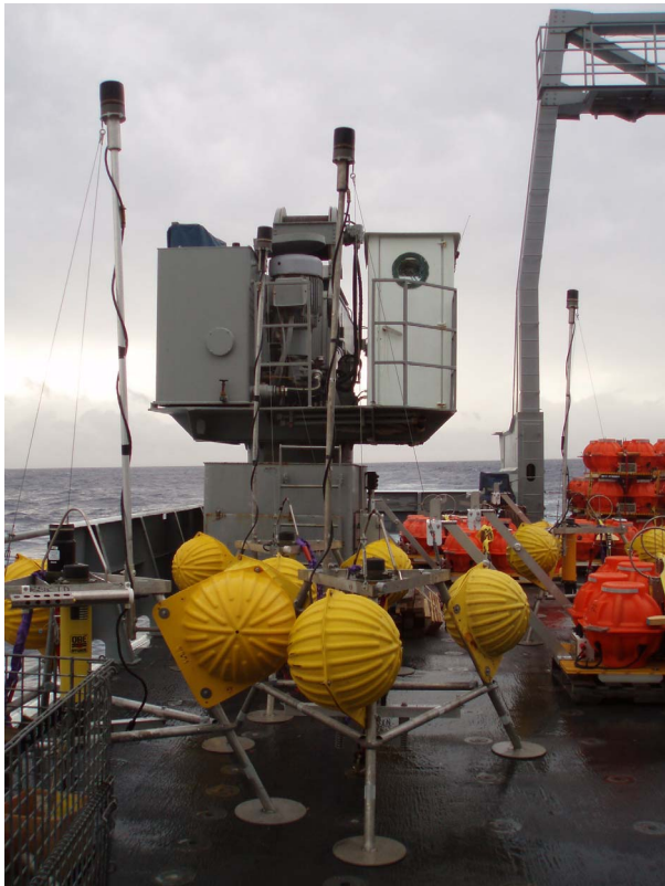
Figure 2. Acoustic ranging tripods on the deck of the R/V Thomas G. Thompson, December 2007.
