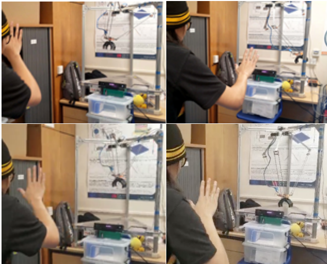
Figure 6. Real-time delta robot control using the hand tracking algorithm.
