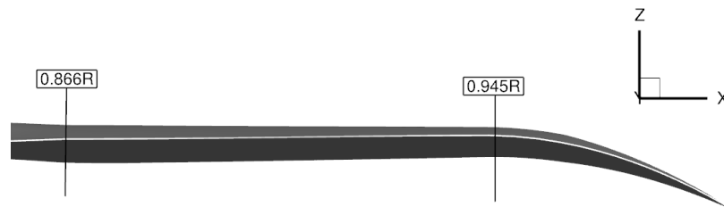
Fig. 15 Geometry of the Langley BERP blade with 15 deg parabolic anhedral, viewed in the streamwise direction.
