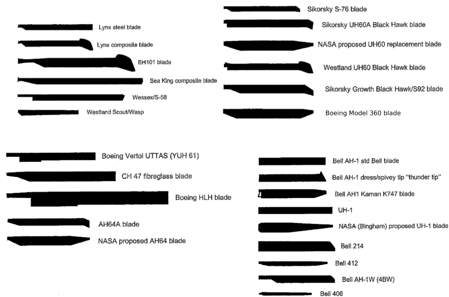
Fig. 1 A wide range helicopter rotor blade planforms showing the variety of used designs [2].
