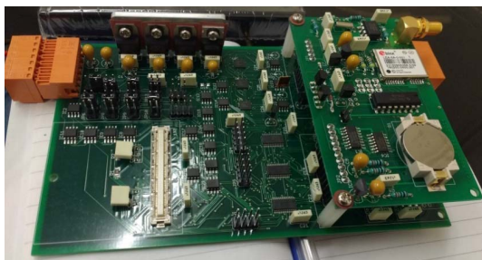
Fig. 2 An image of the custom four-layer electronics board.
