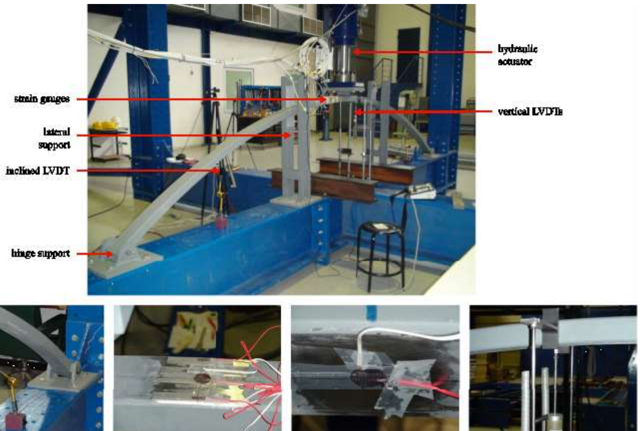
Figure 10: View of the experimental set-up (top) and the measuring devices (bottom) in the following order: inclined LVDT, top flange SG, bottom flange SG, vertical LVDTs.
