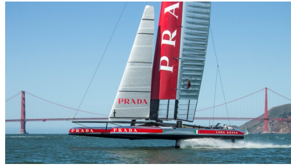
Fig. 1 - America’s Cup catamaran propelled with two-element wingsail.
