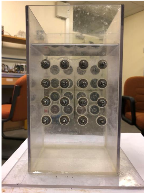
Figure 6.6: Planar Array experimental sensor for 3D image reconstruction: this sensor is designed for different works, in this study, electrodes placed on the single side are used for experiments, and the second array did not involve in this work.
