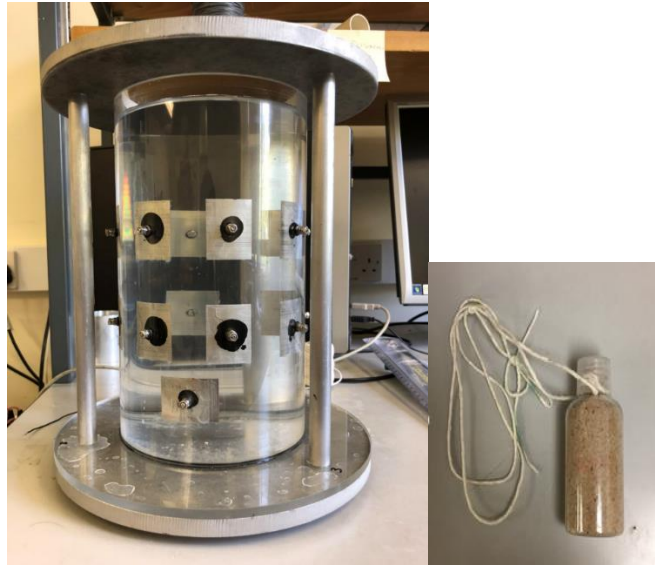
Figure 5.14. Sensor and tested sample of 3D experiments. (a) Phantom of the 3D experimental test: 16 electrodes composed with 2 rings of 8 are utilized for excitation and measurement. The stainless-steel boards are applied to the tank as the main part for the pipe to sit on, which avoid the problem of leaking. (b) Non-conducting inclusion of 3D experiment test: a plastic bottle filled with sands to make sure the inclusion could sink down to the bottle, where tap water was chose as the background and continuous phase.
