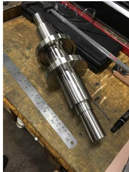
(b) Manufactured shaft according to design.
