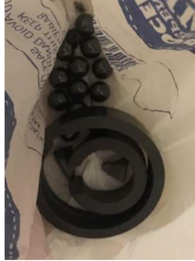
(b) Thermally cycling the bearing cause catastrophic failure.
