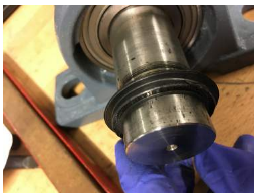
Figure 2.29: Overheating of the seal by running at room temperature causes early failure.
