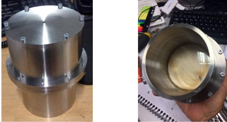
Figure 2.46: Small scale version of sealing technique used for the loss measurement platform. A compression is applied to the glass face which sits on a metal lip greased with apiezon N. An indium seal is used on the external flange to prevent liquid nitrogen or gas ingress.
