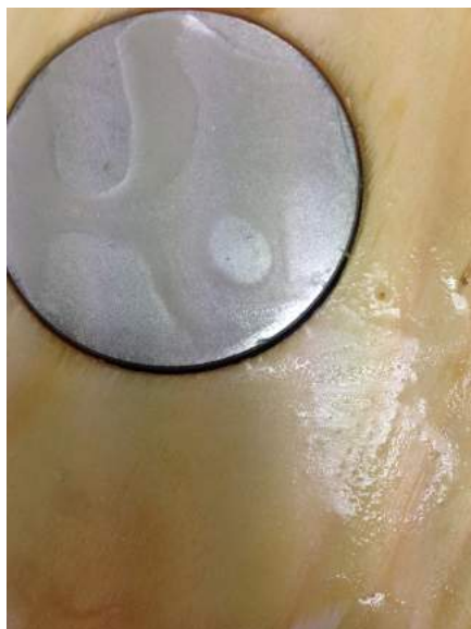
(a) 50 mm NdFeB magnet buried with resin in a 30mm deep wooden bore
