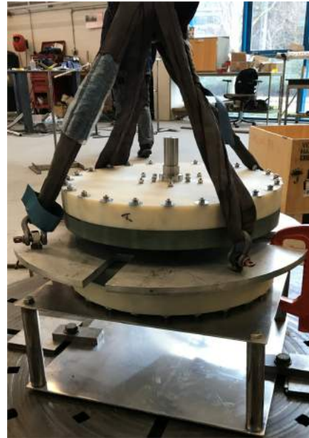
(b) Assembly of the second rotor disc in a controlled manner. The washers on the periphery were used to balance to G-3 spec.
