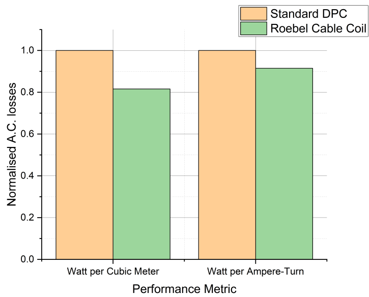
Figure 4.16: A.C. loss comparison between the standard DPC winding and the Roebel coil winding showing improvements at low current loading levels.
