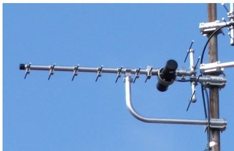
Fig. 1. The 12 elements UHF Yagi-Uda antenna.
