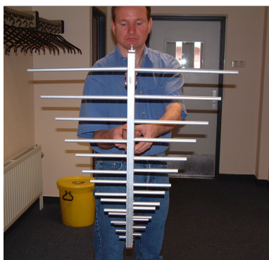
Fig. 2. The 200 MHz to 1 GHz Log-Periodic Dipole Antenna.
