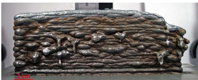
Figure 6 WAAM walls of maraging steel showing degradation with oxide accumulation for torch only shielding [73]
