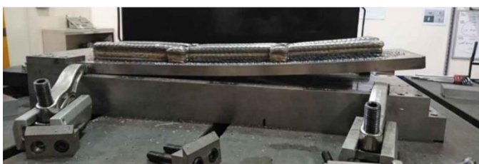
Figure 3 Structural distortion of a WAAM part due to residual stress [42]
