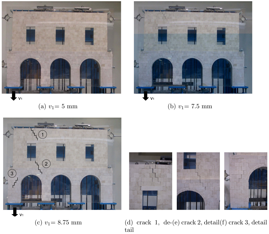
FIG. 8: Test 2: Crack pattern evolution, façade without mortar, test with amplified loading.
