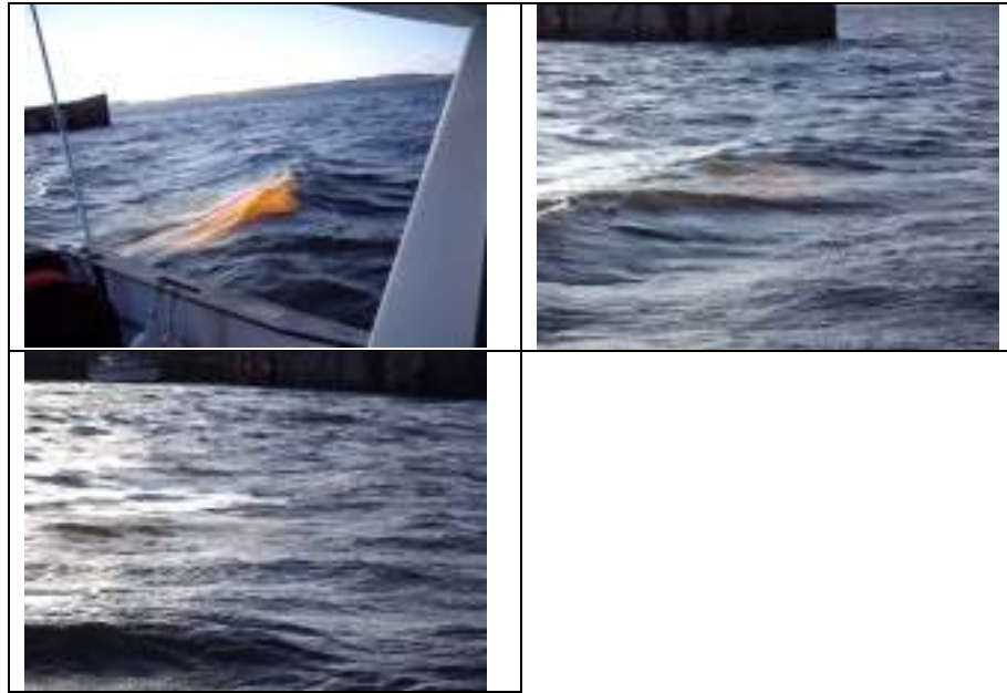
Figure 114 Deployment of tracer off dog leg of break water, tracer movement across harbour mouth in westerly direction
