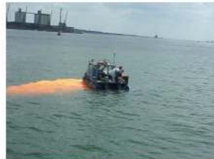
Figure 1. Typical dye tracer being deployed
