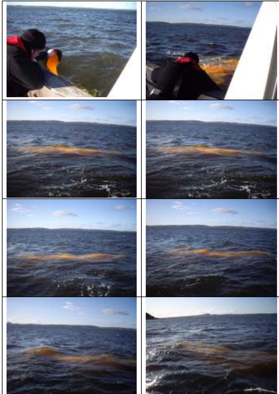
Figure 110 Deployment of tracer off pier point, tracer movement in westerly direction away from harbour.
