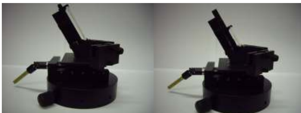
Figure 20 (a) powder sample cell in holder on mount, (b) glass sample in holder on mount
