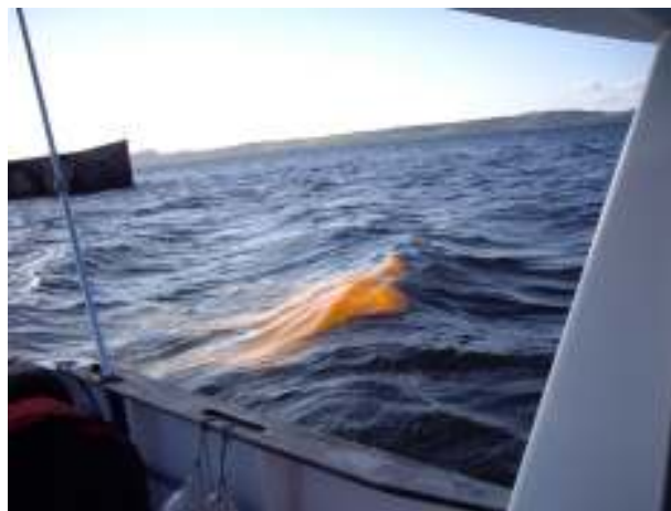
Figure 2 Particulate dye tracer deployment in Bowmore Harbour
