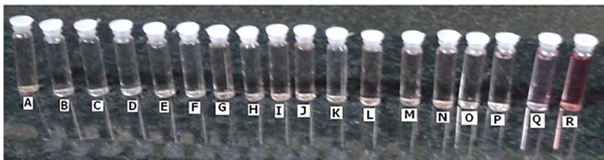
Figure 3. Photographs of color changes of the PH (0.25 \mu\text{M} in 1:10 acetonitrile water in pH 12 Britton–Robinson buffer solution) with different metal ions (3 mL of corresponding metal nitrite solutions of 100 ppm dissolved in water) (a) Probe alone, (b) \text{Pb}^{2+} ions, (c) \text{Cd}^{2+} ions, (d) \text{Ca}^{2+} ions, (e) \text{Ni}^{2+} ions, (f) \text{Mg}^{2+} ions, (g) \text{Zn}^{2+} ions, (h) \text{K}^{+} ions, (i) \text{Fe}^{2+} ions, (j) \text{Fe}^{3+} ions, (k) \text{Al}^{3+} ions, (l) \text{Cr}^{6+} ions, (m) \text{Co}^{2+} ions, (n) \text{Ag}^{+} ions, (o) \text{Cr}^{3+} ions, (p) \text{Mn}^{2+} ions, (q) \text{Hg}^{2+} ions, and (r) \text{Cu}^{2+} ions. [Color figure can be viewed at wileyonlinelibrary.com ]
