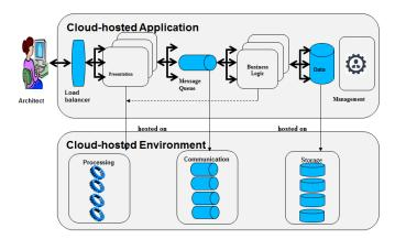
Fig. 1. System Model of a Cloud-hosted Service with multiple groups of components
