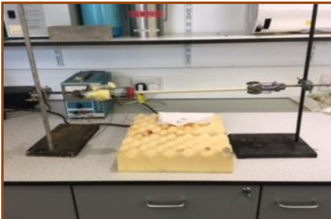
Figure 2-2: Motor powered rotatory dryer
