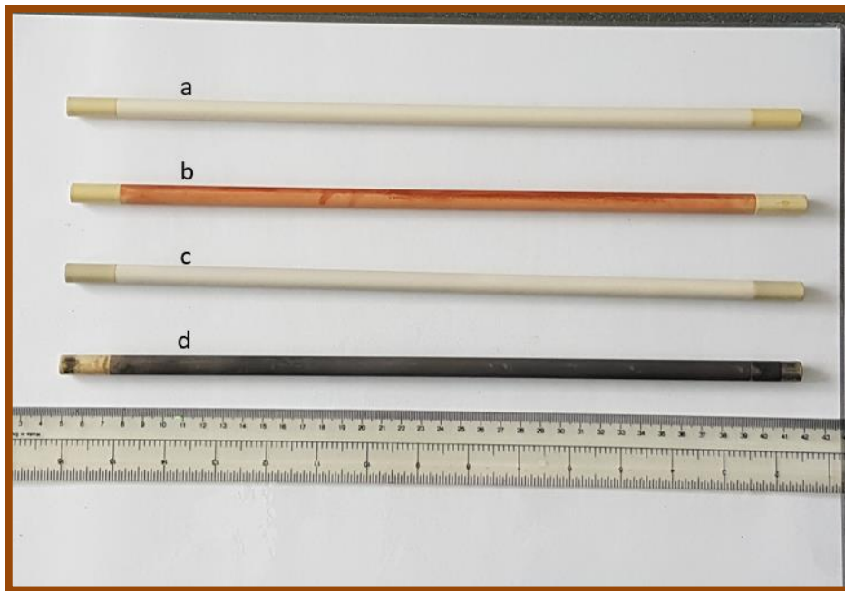
Figure 5-1: pictures of (a) zeolite/ \gamma -alumina membrane, (b) un-activated Rh/ \gamma -alumina membrane, (c) \text{SiO}_2 / \gamma -alumina membrane and (d) activated Rh/ \gamma -alumina membrane
