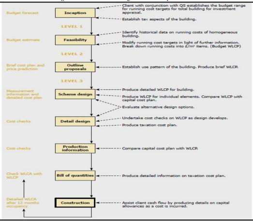
Figure 3.2: Whole life costing and the RIBA plan of work
