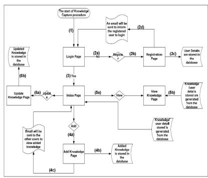
Figure 3.5: Flowchart view of CAPRI.NET approach to knowledge capture and reuse
