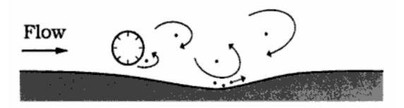
Figure 2.9 Seabed sediment motion due to vortex (Sumer and Fredsoe 2002)
