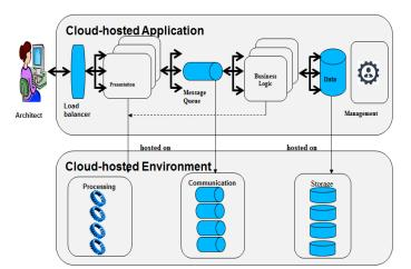
Figure 7.1: System Model of a Cloud-hosted Service with multiple groups of components
