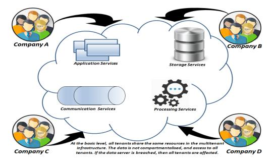
Figure 1.3: Deploying Components of a Cloud-hosted Service in a Multitenant Infrastructure
