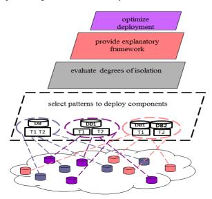
Figure 1.4: A layered architecture for architecting the deployment of cloud-services for guaranteeing multitenancy isolation
