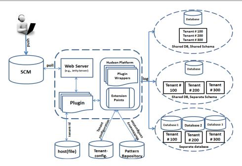
Figure 5.2: Architecture of Multitenancy Isolation at the Data Level.
