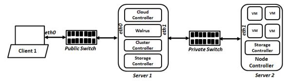
Figure 3.3: Setup of the UEC used for experiments
