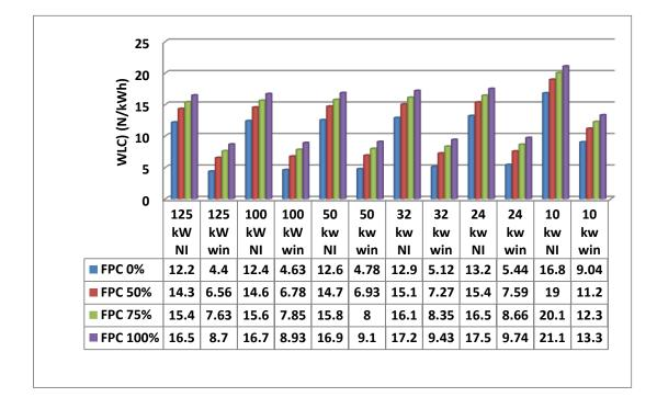
Figure 6.7: Effect of feedstock price fluctuation in WLC of Gasification (wood)
