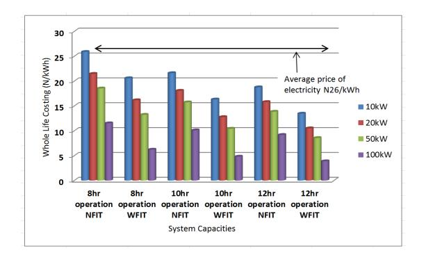
Figure 6.4: WLC of Electricity from Anaerobic Digestion (cattle manure)
