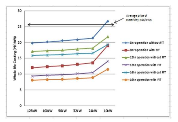
Figure 6.3: WLC of Electricity from Gasification system (Cereal Straw)
