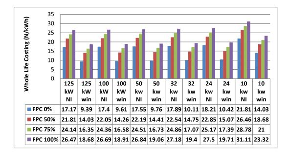
Figure 6.8: Effect of feedstock price fluctuation in WLC in Gasification (cereal straw)
