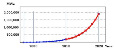
Figure 2.5: Total worldwide installed wind capacity 1997–2020 (MWe): Development & Forecast (Sopian et al. 2011).
