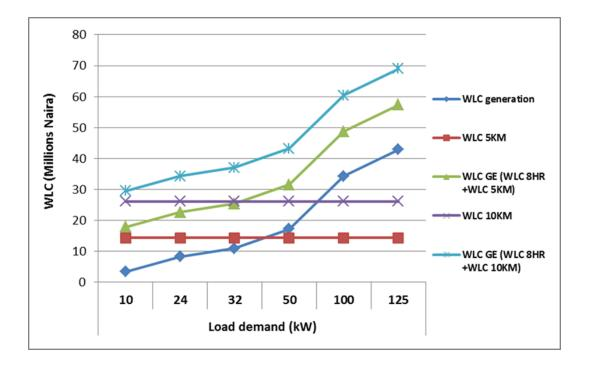
Figure 6.9: Effect of WLC of Electricity Generation over WLC of GE system
