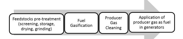
Figure 3.2: Gasification Processes for Electricity Generation (Adopted from: Demirbas 2009; Bocci et al. 2014; IRENA 2012)
