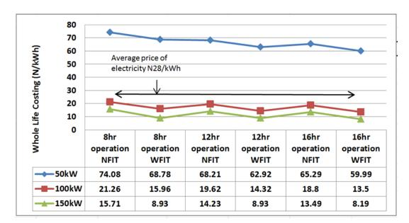
Figure 6.1: WLC/kWh of Electricity from Direct Combustion (wood fuel)
