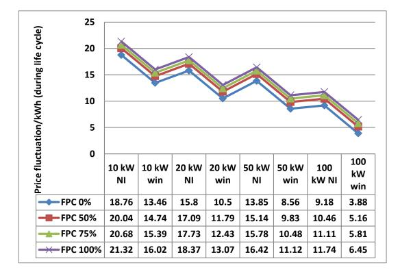
Figure 6.6: Effect of feedstock price fluctuation in WLC of Anaerobic Digestion
