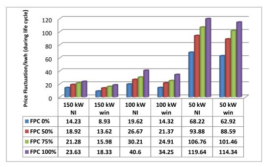
Figure 6.5: Effect of feedstock price fluctuation in WLC of Direct Combustion
