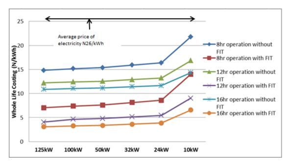
Figure 6.2: WLC of Electricity from Gasification system (wood fuel)
