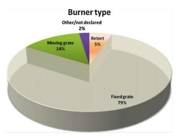
Figure 3.4: Burners types as applied in the Industry (Miguez et al. 2012)
