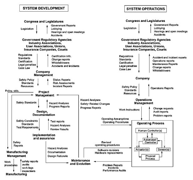
Figure 1-1 : General form of a model of socio-technical control (Leveson, 2004)
