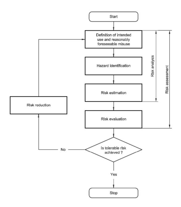
Figure 1-4: The iterative process of risk management (ISO guide, 2012)
