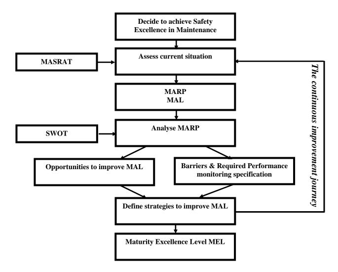
Figure 1-20: A framework for safety excellence in the maintenance system of oil and gas asset
