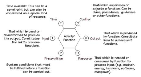
Figure 1-2 : The FRAM functional unit, module (Hollnagel, 2010a)
