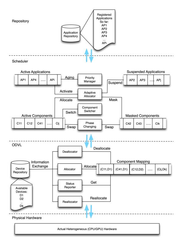
Figure 4.5: An architectural view of the Proposed OpenCL Scheduler and its relationship with ODVL and application registry. The blue arrows represents the communication mechanism. The solid lines connecting a module to a queue represent the type of operation applied by the module in the specified queue
