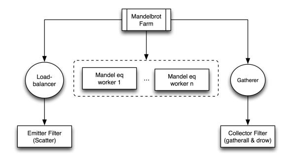
Figure 6.2: The structural composition of components for the Mandelbrot application in FastFlow visualised by structural tree notation
