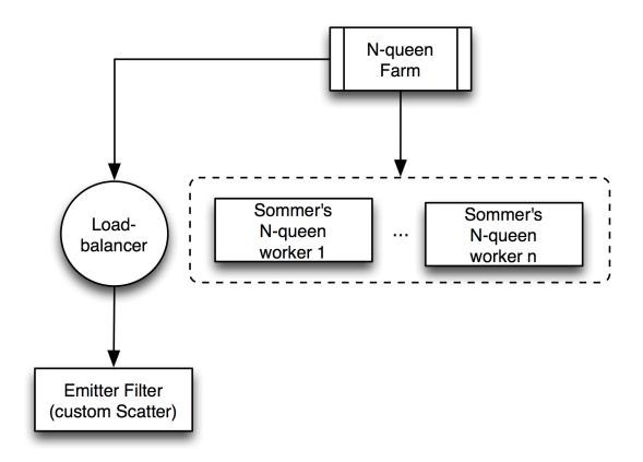
Figure 6.6: The structural composition of components for the *N*-queen application in Fast-Flow visualised by structural tree notation An instance of ff\_loadbalancer with a custom filter function has been applied. The CustomScatter function adjusts the board until depth K in the tree and then sends it to the workers to complete it.
