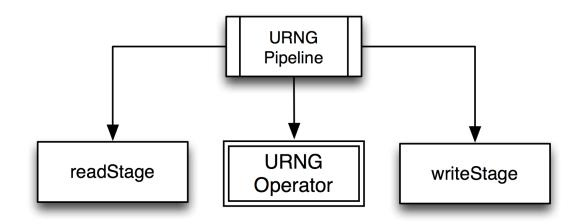
Figure 5.4: The structural composition of components for the URNG application in HFast-Flow visualised by structural tree notation
