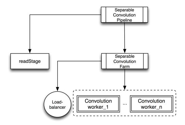
Figure 5.6: The structural composition of components for the Simple Convolution application in HFastFlow visualised by structural tree notation
