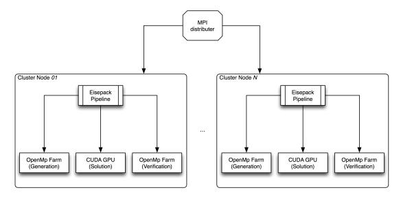
Figure 6.7: The structural composition of components for the EISPACK application encapsulating the FastFlow pipeline patter. It is visualised by structural tree notation. The application is composed of a three-level hierarchy of skeletons, consisting of a distributed farm of MPI workers at the top-level that contains nested pipeline workers with nested OpenMP farm stages and a GPU stage.
