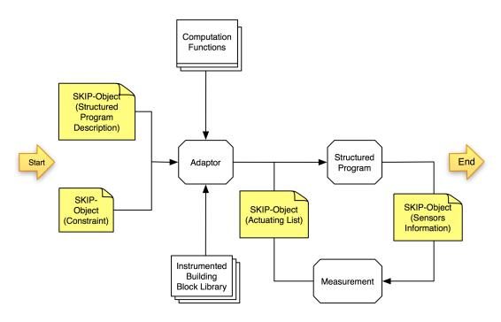
Figure 3.1: Schematic view of construction and execution of a structured program using SKIP compliant autonomic behavioural system
