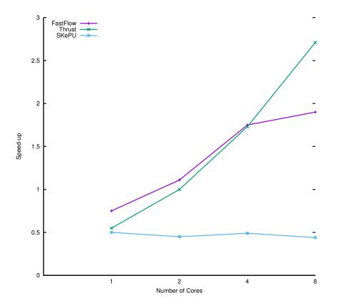
Figure 6.10: Speed-up graph for *N*-body simulation using FastFlow, Thrust and SkePU (Problem size: 1024 bodies)
