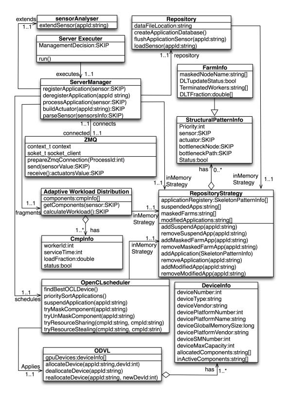
Figure 4.4: A class diagram representing the DSRI Server and its relationship with the embedded coordination engines.
