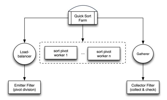
Figure 6.3: The structural composition of components for the quick sort application in Fast-Flow visualised by structural tree notation
