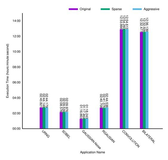
Figure 5.7: The upper-bound overhead of performance metrics tracing over the HFastFlow framework on a node of the Xookik cluster for image processing applications.
