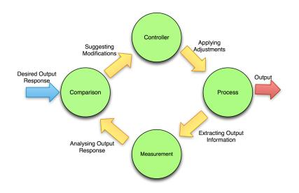
Figure 2.1: Feedback control system
