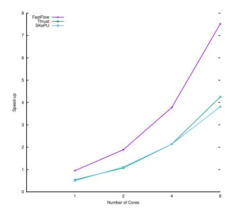
Figure 6.12: Speed-up graph for *N*-body simulation using FastFlow, Thrust and SkePU (Problem size: 65536 bodies)
