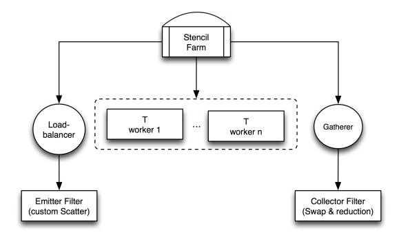
Figure 6.5: The structural composition of components for the stencil application in FastFlow visualised by structural tree notation
