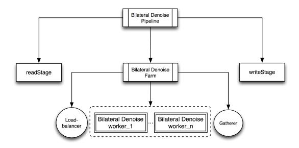
Figure 5.2: The structural composition of components for the Bilateral Denoise application in HFastFlow visualised by structural tree notation
