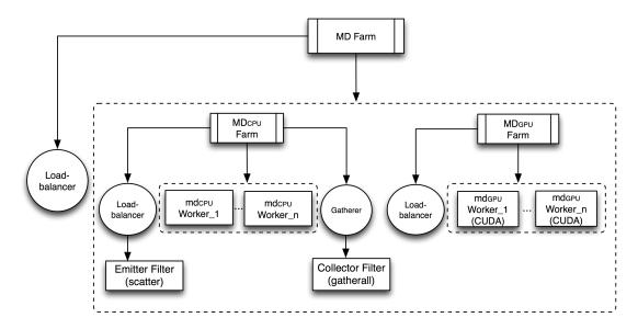
Figure 6.9: The structural composition of components for the *MD* application in FastFlow visualised by structural tree notation
