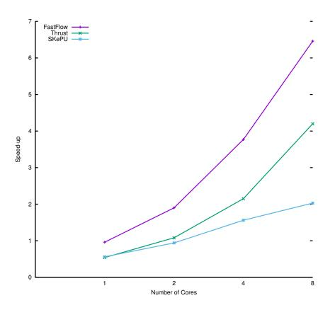
Figure 6.11: Speed-up graph for *N*-body simulation using FastFlow, Thrust and SkePU (Problem size: 8192 bodies)
