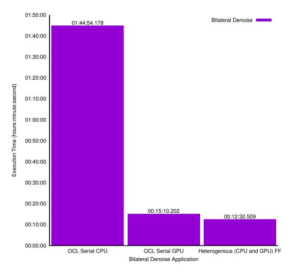
Figure 5.8: Execution of Bilateral denoise using OpenCL back-end
