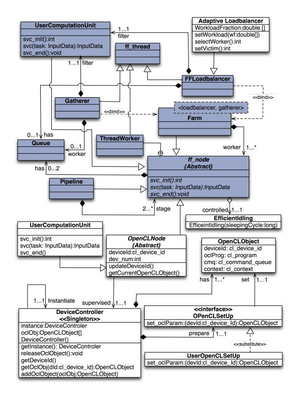
Figure 4.1: A UML class diagram for instrumented FastFlow. Existing classes in FastFlow have been marked in grey
