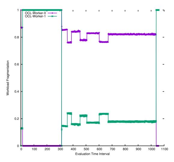
Figure 5.18: The visual demonstration of the concurrent execution intervals for the sobel filter and convolution applications where the priority of sobel filter application is higher than the priority of the convolution application
