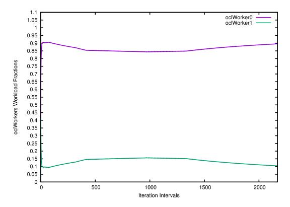
Figure 5.12: The variation of workload distribution for CPU/GPU workers for different input stream sizes on a node of the Xookik cluster using the average policy for bilateral denoise
