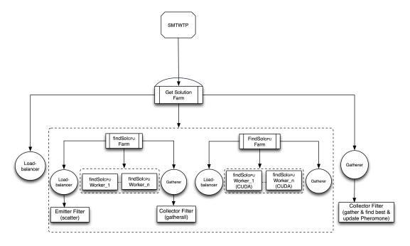
Figure 6.8: The structural composition of components for the *SMTWTP* application in Fast-Flow visualised by structural tree notation
