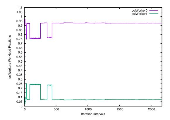
Figure 5.11: The variation of workload distribution for CPU/GPU workers for different input stream sizes on a node of the Xookik cluster using the ad-hoc policy for bilateral denoise
