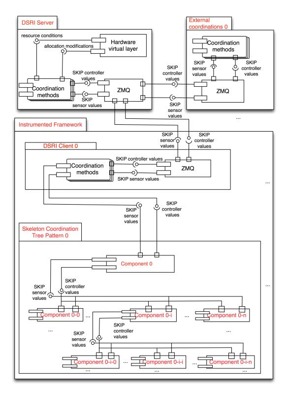
Figure 4.6: A component diagram representing the physical view of the autonomous behavioural framework
