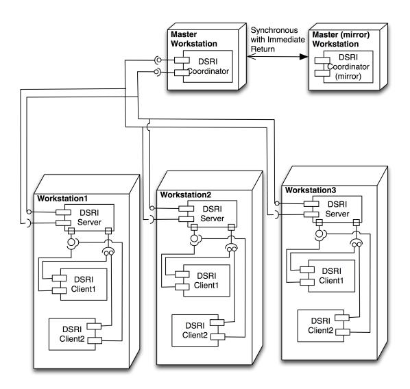
Figure 7.1: Deployment diagram for distributed PEI
