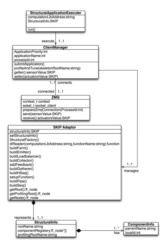
Figure 4.2: A class diagram representing the DSRI client and its relationship with client side objects
