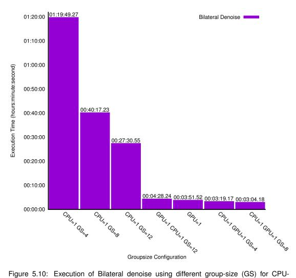
Figure 5.10: Execution of Bilateral denoise using different group-size (GS) for CPUallocated OpenCL workers on a node of the Xookik cluster. The number of CPU or GPU workers used for each execution is demonstrated in the caption of each column.
