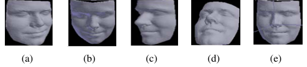
Figure 8. 3D facial scan images representing 4 different poses (a) +30 degree around the y-axis (b) rotated by 30 degree around the z-axis (c) rotated by -30 degree around the y-axis (d) rotated by -30 degree around the x-axis and (e) aligned within the Cartesian coordinate with the nose tip residing at the origin as detailed in section 4.
