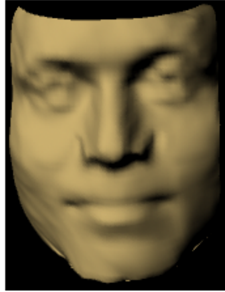
Figure 6. PDE facial surface with an increased mesh resolution, the surface is controlled by the same set of boundary curves shown in Figure 5 (a).
