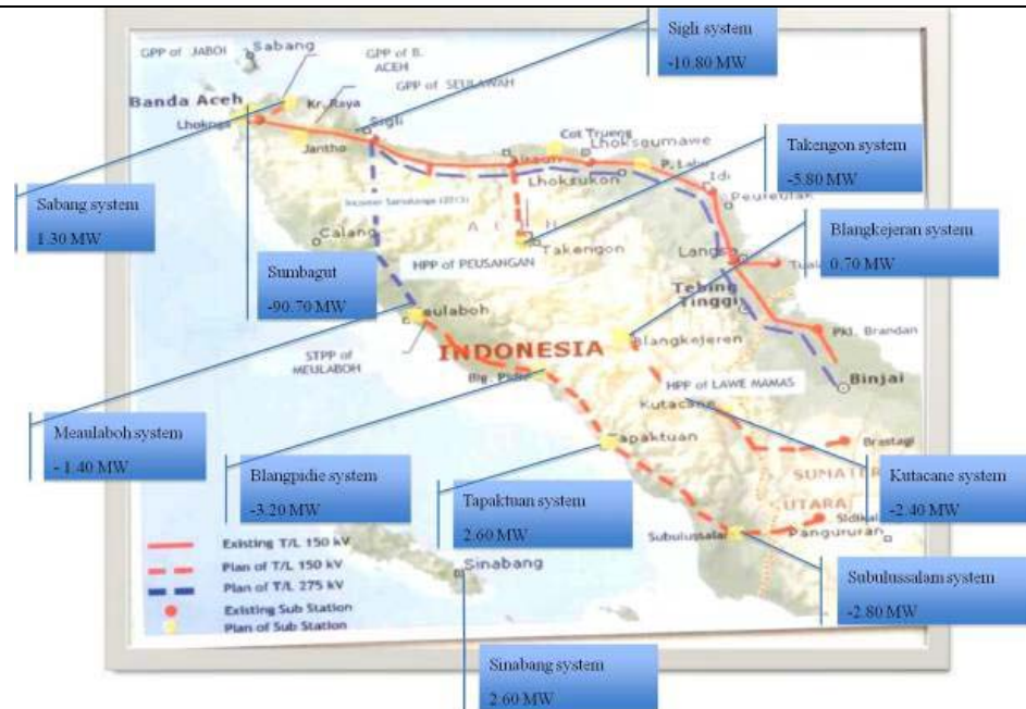
Figure 4-4: Deficits for Isolated Systems in Aceh, Modified from Ministry of Energy and Mineral Resources (ESDM) 2009. Master Plan ketenagalistrikan 2010-2014, page 17.
