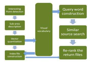
Figure 2.8: The basic architecture of CBVR based on bag of visual word
