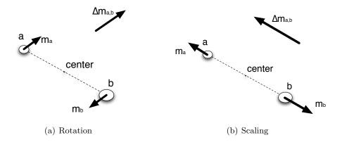
Figure 3.11: The relative motion can be caused by the affine transformation of visual object.
