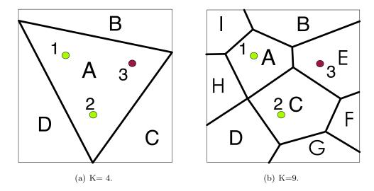
Figure 5.1: Two types of quantization error. K is the size of visual vocabulary.
