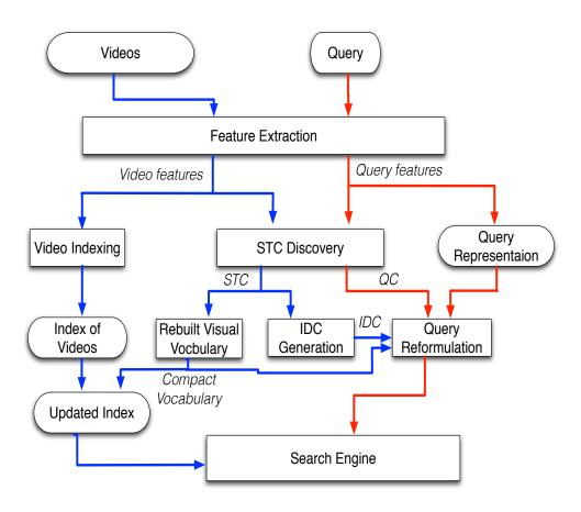
Figure 6.1: The Architecture of the prototype CBVR System based on the STC
