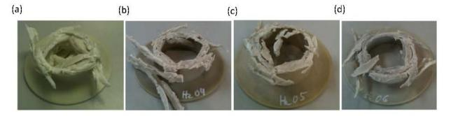
Figure 3: Static collapse mode of PA6 composites (a) PA/GF (b) PA/GF/SiO<sub>2</sub> (c) PA/GF/MMT (d) PA/GF/GS.
