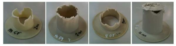
Figure 2: Dynamic collapse mode of PA6 composites (a) PA/GF (b) PA/GF/SiO<sub>2</sub> (c) PA/GF/MMT (d) PA/GF/GS
