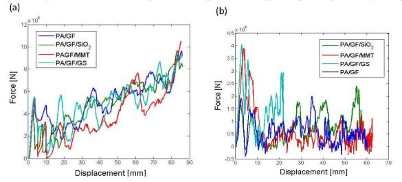
Figure 1. Load-displacement curves (a) static (b) dynamic.
