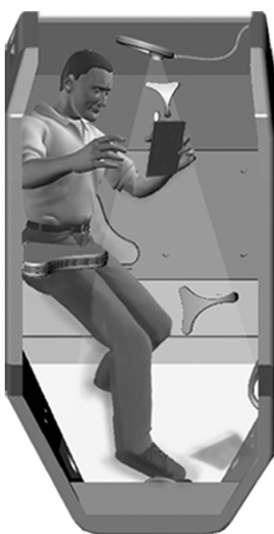
Figure 15: CQ System Overview #1 - A crewmember is shown in an active reading position, bracing between the lower surfaces of the CQ shell. A list of parts shows the combination for this CQ arrangement.
