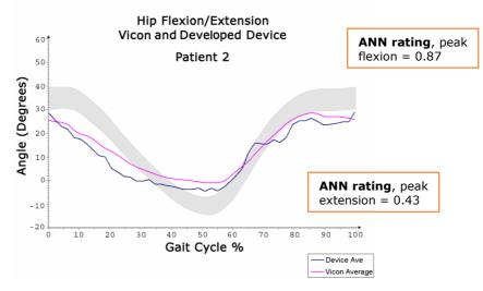
*Figure 6.8.3: Patient 2 hip flexion/extension waveform from developed device, Vicon system, and with ANN key landmark ratings at peak/trough values*
