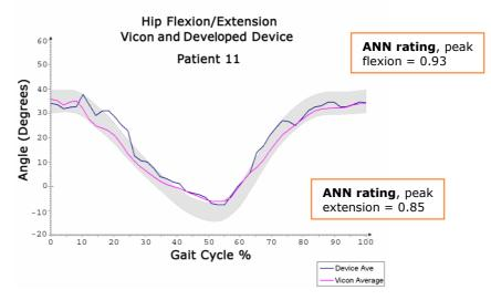
*Figure 6.8.21: Patient 11 hip flexion/extension waveform from developed device, Vicon system, and with ANN key landmark ratings at peak/trough values*
