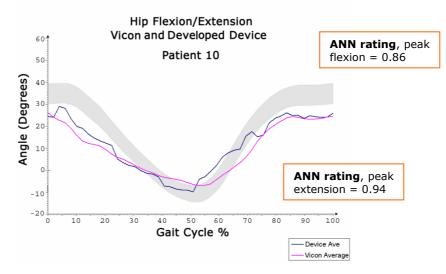
*Figure 6.8.19: Patient 10 hip flexion/extension waveform from developed device, Vicon system, and with ANN key landmark ratings at peak/trough values*
