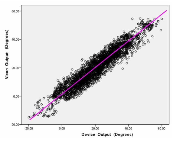
*Figure 7.4.1.1: Scatter plot of device output with respect to Vicon, with centre of mass shown, for hip flexion/extension*
