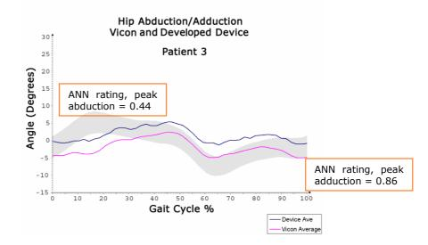
*Figure 6.8.6: Patient 3 hip abduction/adduction waveform from developed device, Vicon system, and with ANN key landmark ratings at peak/trough values*
