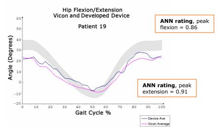
*Figure 6.8.37: Patient 19 hip flexion/extension waveform from developed device, Vicon system, and with ANN key landmark ratings at peak/trough values*
