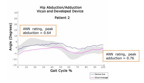
*Figure 6.8.4: Patient 2 hip abduction/adduction waveform from developed device, Vicon system, and with ANN key landmark ratings at peak/trough values*
