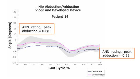
Figure 6.8.32: Patient 16 hip abduction/adduction waveform from developed device, Vicon system, and with ANN key landmark ratings at peak/trough values
