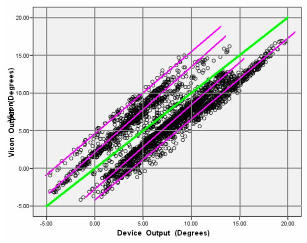
*Figure 7.4.1.3: Gridline enhanced scatter plot of device output with respect to Vicon for hip abduction/adduction*
