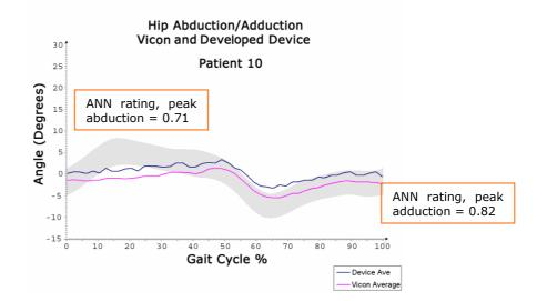
Figure 6.8.20: Patient 10 hip abduction/adduction waveform from developed device, Vicon system, and with ANN key landmark ratings at peak/trough values
