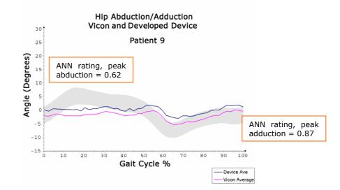
*Figure 6.8.18: Patient 9 hip abduction/adduction waveform from developed device, Vicon system, and with ANN key landmark ratings at peak/trough values*
