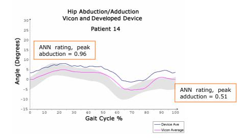
*Figure 6.8.28: Patient 14 hip abduction/adduction waveform from developed device, Vicon system, and with ANN key landmark ratings at peak/trough values*
