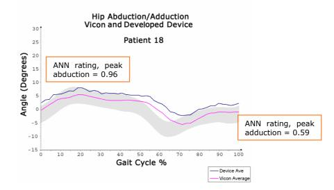
*Figure 6.8.36: Patient 18 hip abduction/adduction waveform from developed device, Vicon system, and with ANN key landmark ratings at peak/trough values*
