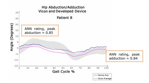
*Figure 6.8.16: Patient 8 hip abduction/adduction waveform from developed device, Vicon system, and with ANN key landmark ratings at peak/trough values*
