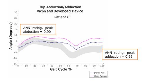
*Figure 6.8.12: Patient 6 hip abduction/adduction waveform from developed device, Vicon system, and with ANN key landmark ratings at peak/trough values*
