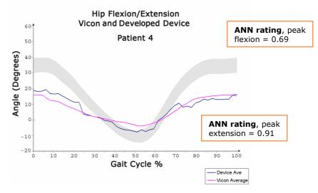
*Figure 6.8.7: Patient 4 hip flexion/extension waveform from developed device, Vicon system, and with ANN key landmark ratings at peak/trough values*
