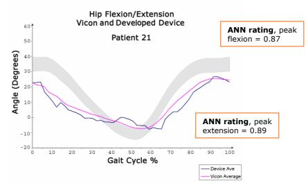
*Figure 6.8.41: Patient 21 hip flexion/extension waveform from developed device, Vicon system, and with ANN key landmark ratings at peak/trough values*
