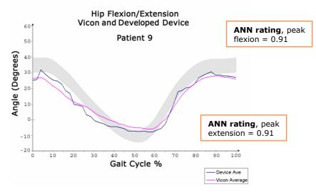
*Figure 6.8.17: Patient 9 hip flexion/extension waveform from developed device, Vicon system, and with ANN key landmark ratings at peak/trough values*
