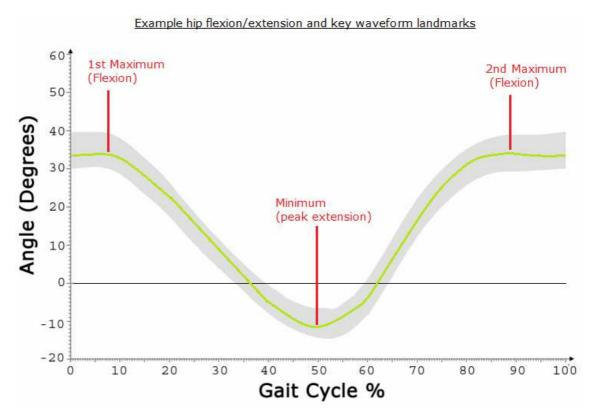
Figure 6.6.1: Hip flexion/extension waveform landmarks of interest
