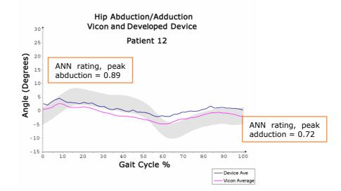
Figure 6.8.24: Patient 12 hip abduction/adduction waveform from developed device, Vicon system, and with ANN key landmark ratings at peak/trough values
