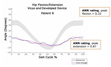
*Figure 6.8.15: Patient 8 hip flexion/extension waveform from developed device, Vicon system, and with ANN key landmark ratings at peak/trough values*
