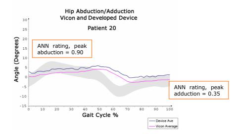
Figure 6.8.40: Patient 20 hip abduction/adduction waveform from developed device, Vicon system, and with ANN key landmark ratings at peak/trough values
