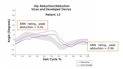
Figure 6.8.26: Patient 13 hip abduction/adduction waveform from developed device, Vicon system, and with ANN key landmark ratings at peak/trough values
