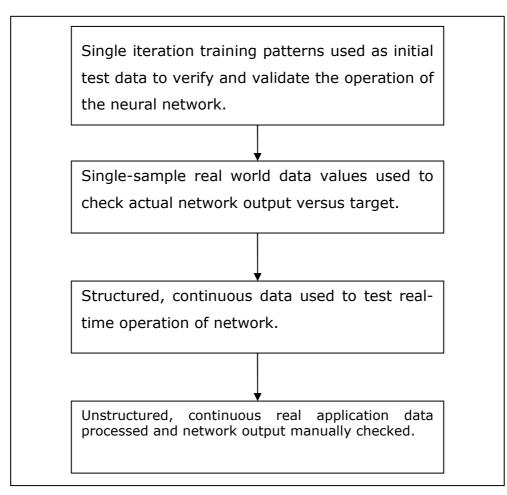
Figure 5.7.1: Software testing overview
