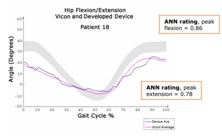
*Figure 6.8.35: Patient 18 hip flexion/extension waveform from developed device, Vicon system, and with ANN key landmark ratings at peak/trough values*
