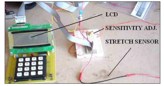
Figure 2: Test apparatus for stretch sensor
