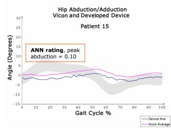
*Figure 7.3.2: Patient 15 hip abduction/adduction waveform from developed device, Vicon system, and with ANN key landmark ratings at peak/trough values*
