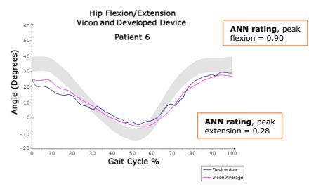
*Figure 6.8.11: Patient 6 hip flexion/extension waveform from developed device, Vicon system, and with ANN key landmark ratings at peak/trough values*
