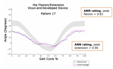
*Figure 6.8.33: Patient 17hip flexion/extension waveform from developed device, Vicon system, and with ANN key landmark ratings at peak/trough values*
