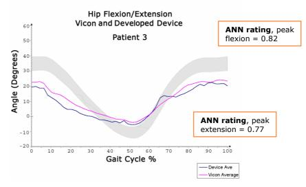
*Figure 6.8.5: Patient 3 hip flexion/extension waveform from developed device, Vicon system, and with ANN key landmark ratings at peak/trough values*
