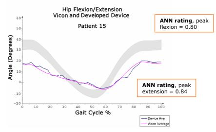
*Figure 6.8.29: Patient 15 hip flexion/extension waveform from developed device, Vicon system, and with ANN key landmark ratings at peak/trough values*
