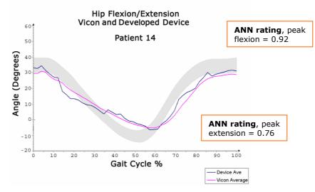
*Figure 6.8.27: Patient 14 hip flexion/extension waveform from developed device, Vicon system, and with ANN key landmark ratings at peak/trough values*
