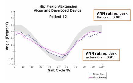
*Figure 6.8.23: Patient 12 hip flexion/extension waveform from developed device, Vicon system, and with ANN key landmark ratings at peak/trough values*
