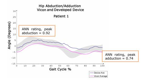
*Figure 6.8.2: Patient 1 hip abduction/adduction waveform from developed device, Vicon system, and with ANN key landmark ratings at peak/trough values*
