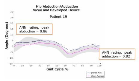
*Figure 7.5.3: Patient 19 hip abduction/adduction waveform from developed device, Vicon system, and with ANN key landmark ratings at peak/trough values*
