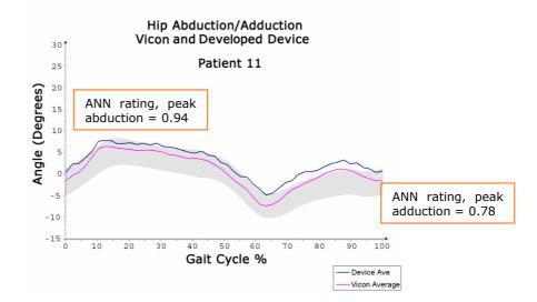
Figure 6.8.22: Patient 11 hip abduction/adduction waveform from developed device, Vicon system, and with ANN key landmark ratings at peak/trough values
