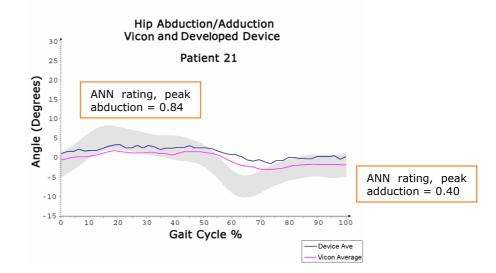
Figure 6.8.42: Patient 21 hip abduction/adduction waveform from developed device, Vicon system, and with ANN key landmark ratings at peak/trough values
