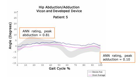
*Figure 6.8.10: Patient 5 hip abduction/adduction waveform from developed device, Vicon system, and with ANN key landmark ratings at peak/trough values*
