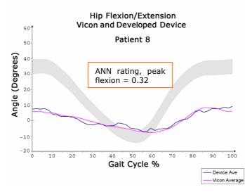
*Figure 7.3.1: Patient 8 hip flexion/extension waveform from developed device, Vicon system, and with ANN key landmark ratings at peak/trough values*
