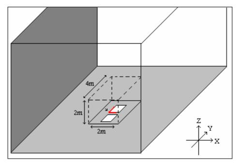
Figure 3.9.1.1: Force plates, 'L'-frame placement and calibration volume
