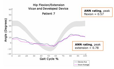
*Figure 6.8.13: Patient 7 hip flexion/extension waveform from developed device, Vicon system, and with ANN key landmark ratings at peak/trough values*
