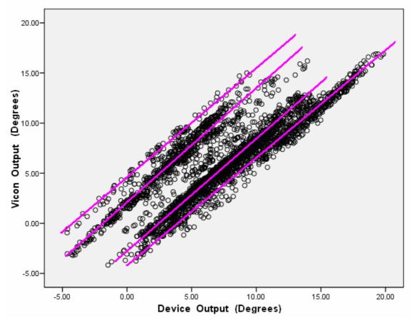
*Figure 7.4.1.2: Scatter plot of device output with respect to Vicon for hip abduction/adduction*
