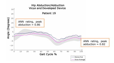
*Figure 6.8.38: Patient 19 hip abduction/adduction waveform from developed device, Vicon system, and with ANN key landmark ratings at peak/trough values*
