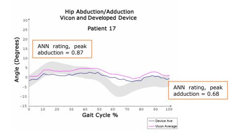
Figure 6.8.34: Patient 17 hip abduction/adduction waveform from developed device, Vicon system, and with ANN key landmark ratings at peak/trough values
