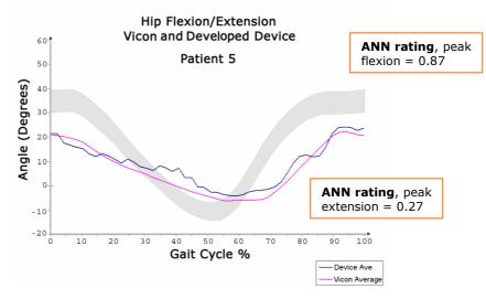
*Figure 6.8.9: Patient 5 hip flexion/extension waveform from developed device, Vicon system, and with ANN key landmark ratings at peak/trough values*
