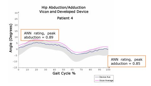
*Figure 6.8.8: Patient 4 hip abduction/adduction waveform from developed device, Vicon system, and with ANN key landmark ratings at peak/trough values*
