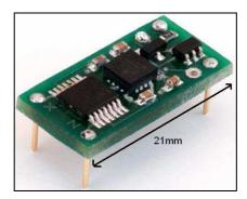
*Figure 4.3.1: The Dimension Engineering 3-axis accelerometer Source: Dimension Engineering data sheet*
