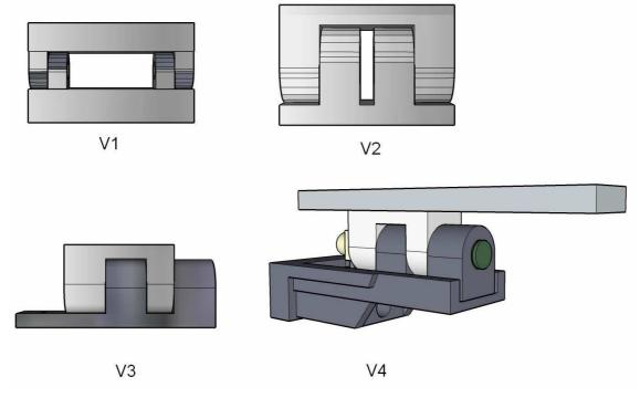
Figure 8: The evolution of the medial/lateral hinge
