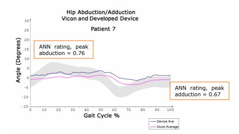
*Figure 6.8.14: Patient 7 hip abduction/adduction waveform from developed device, Vicon system, and with ANN key landmark ratings at peak/trough values*
