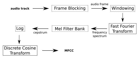
Figure 5.2: The MFCC Algorithm
