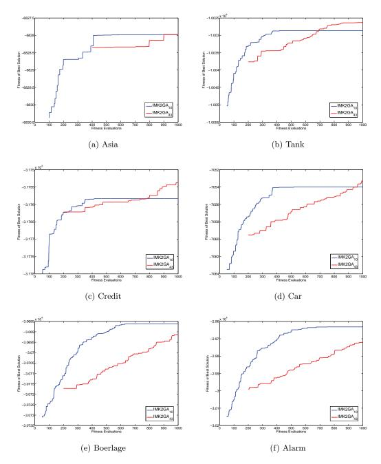
Figure 4.1: Evolution of the fitness of the best solution in  $IMK2GA_{10}$  and  $IMK2GA_{43}$  on all benchmark problems
