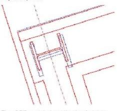
Figure 2 Differences in size and location of columns. Electronic overlay comparing two different drawings that had been approved for construction (architect's drawing - red, structural engineer's – blue). Source: www.productioninformation.org/images/final/FigS12.gif)
