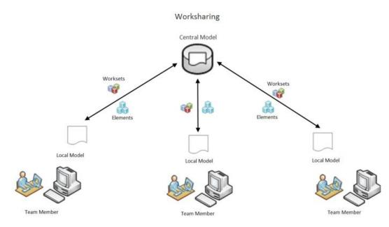
Figure 9 Diagram of Central file and Worksets, courtesy Autodesk WikiHelp
