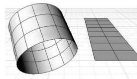
Developable surfaces can be formed by rolling a flat sheet of material without stretching it.
