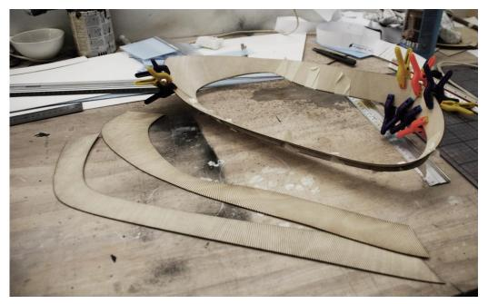
A working model, showing that the developed shapes assemble into the correct form
