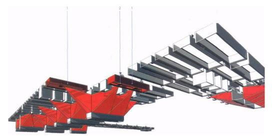
Figure 27 The BIM model was used to position the ceiling-mounted projectors accurately, courtesy of Architects Journal 23/07/09
