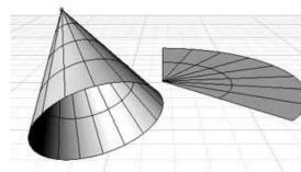
A developed surface is the consequence of unrolling a form where a modifier has been applied.
