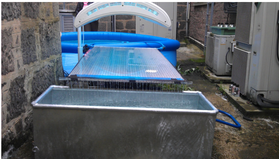
Figure 4.4: Reactor in operation with 40 to 50 cm distance of illumination
