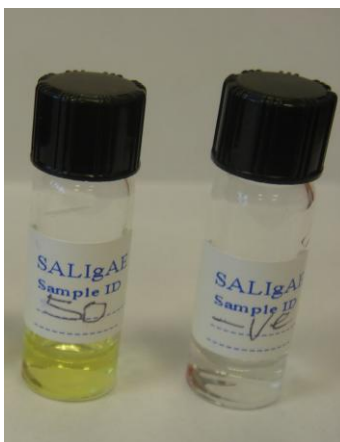
Figure 3.3: SALigAE vial tests showing from left to right, positive and negative test results respectively (photo taken in house)
