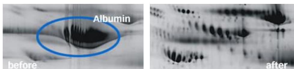
Figure 4.2: A 2D gel image showing a human serum sample before and after treatment with Vivapure ® Anti HSA/IgG kit removing Albumin. (source: Sartorius Stedim Biotech).
