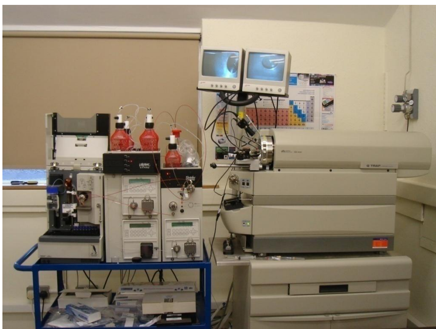
Figure 2.8: A Photograph to show the UltiMate nanoLC system and Q trap Quadrupole MS (photograph taken in house).
