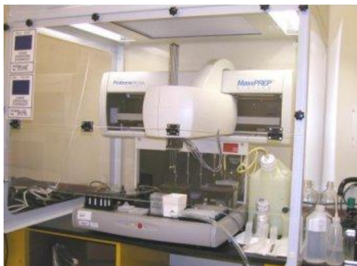
Figure 2.7: A Photograph to show the Mass prep automated liquid handling system (Rowett Institute of Nutrition and Health)
