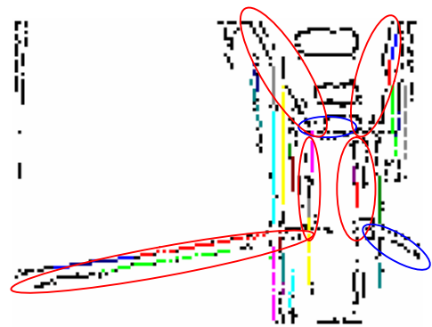
Figure 5.19 Lines and sub-lines found in image3 with T=150 (a) Lines (b) Sub-lines
