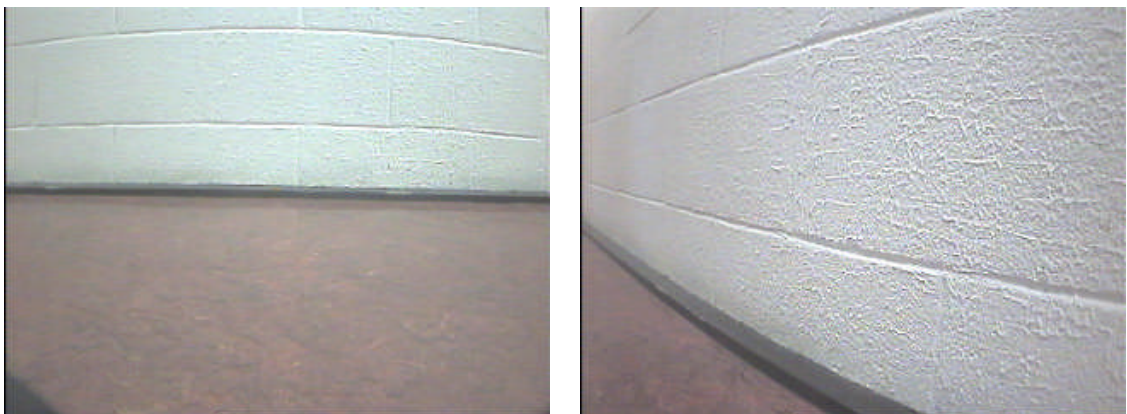
Figure 1. 2 Contrast between floor and wall (a) with robot 'looking' across the corridor (b) with robot at an angle to the corridor
