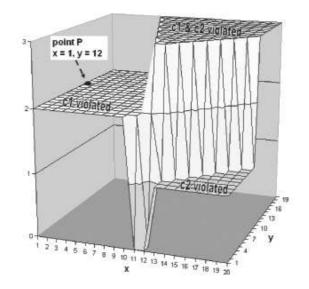
Fig. 4. Effect of constraint weight increase on the cost landscape for the CSP in Figure 3.
