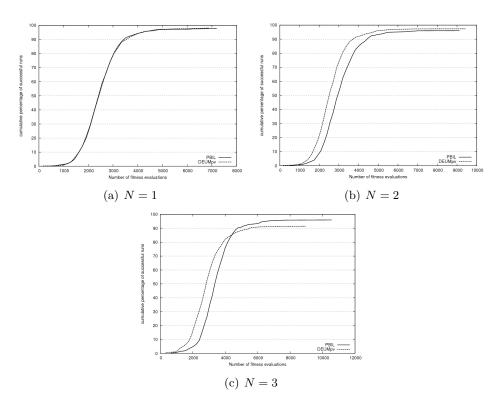
**Figure 5.7:** Experimental results in the form of RLD comparing  $\text{DEUM}_{pv}$  and PBIL for 20-bit binary representation Schaffer f6 function. For both algorithms population size was 160, learning rate was 0.1 and selection size, N, was 1 for (a), 2 for (b) and 3 for (c).
