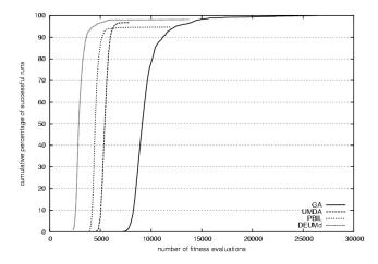
**Figure 6.3:** Experimental results in the form of RLD showing, for each algorithm running on the 180 bit Plateau problem, the cumulative percentage of successful runs that terminated within a certain number of function evaluations
