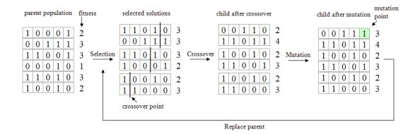
Figure 2.5: A simulation of a simple GA iteration
