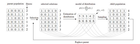
Figure 2.8: A simulation of variation by means of estimation of distribution and sampling
