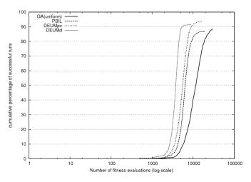
Figure 6.7: RLD for DEUM<sub>d</sub> in comparison to DEUM<sub>pv</sub> and other univariate EDAs, showing, for each algorithm running on the 20-bit gray code representation of Schaffer f6 function, the cumulative percentage of successful runs that terminated within a certain number of function evaluations
