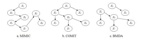
Figure 2.14: Graphical representation of linkage with pair-wise interaction between variables
