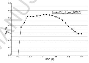
Fig. 12. Voltage variation difference for different discharging currents
