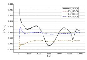
Fig. 19. SOC estimation error under different working conditions
