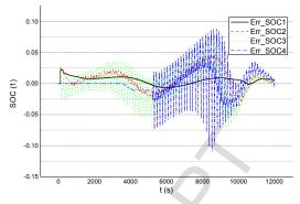
Fig. 17. SOC estimation error under different working conditions
