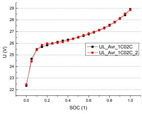
Fig. 9.OCV-SOC curve fitting effect analysis
