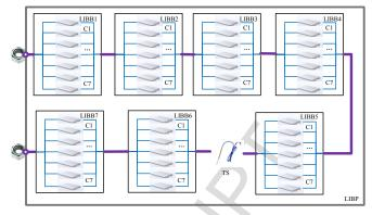
Fig. 1. The representative structure of the lithium-ion battery packs
