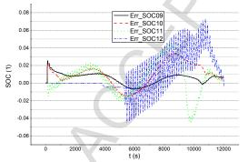
Fig. 21. SOC estimation error under different working conditions
