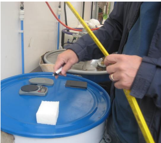
Figure 11. Quality check of the foam
