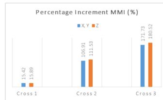
The MMI increases respect to state-of-art shape in all three new shapes. The figure shows better this result by the percentage increment of the MMI respect to the state-of-art circular shape.
