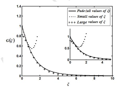
Fig. 2(b). Comparison of our tangential velocity component  $G(\xi)$  (Padé approximation Eq. (C5)) *versus* the dimensionless distance  $\xi$  with small (Eq. (2)) and long solution (Eq. (8)).
