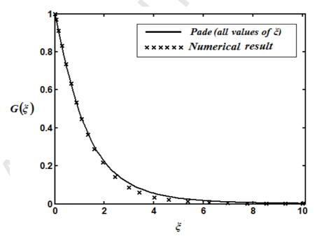
Fig. 1(b). Dimensionless tangential velocity component  $G(\xi)$  versus the dimensionless distance profile. The key to the graph: solid line represents Eq. (C5) and the dotted line represents the numerical [3].
