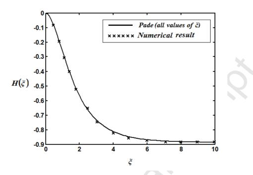
Fig. 1(c). Dimensionless axial velocity component  $H(\xi)$  versus the dimensionless distance profile. The key to the graph: solid line represents Eq. (D5) and the dotted line represents the numerical [3].
