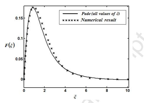
Fig. 1(a). Dimensionless radial velocity component  $F(\xi)$  versus the dimensionless distance profile. The key to the graph: solid line represents Eq. (B10) and the dotted line represents the numerical [3].
