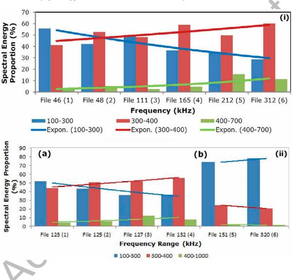
**Fig. 11.** Averaged spectral energy: (a) for identified DCB experimental AE source: adhesive failure, (b) for identified DCB experimental AE source: adhesive stressing, (c) for identified 3-ENF experimental AE source: (potential) adhesive failure, and (d) for 3-ENF experimental AE source: elastic/plastic deformation of material [figures appear in colour *in* the online version].
