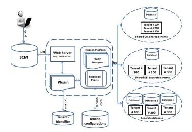
Fig. 2. Multitenancy Isolation Architecture for Cloud-hosted Applications.
