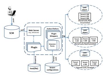
Fig. 3. Multitenancy Isolation Architecture for Cloud-hosted Applications.
