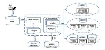
Figure 2. Multitenancy Data Isolation Architecture
