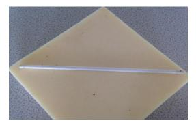
Figure 1: Porous tubular alumina support.
