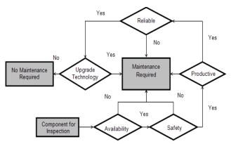
Figure 1 A Maintenance Decision model to check the need for maintenance implementation
