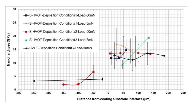
**Figure 13**, Nanohardness results of coating substrate systems deposited under deposition conditions # 1, 2, 3. Zero at x-axis represents the location of coating-substrate interface and the distances represented are measured from this interface.
