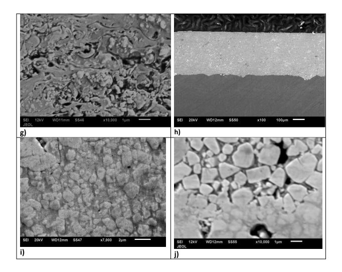
**Figure 3**, SEM observations of deposited coatings, a) surface of as-deposited coatings under spraying condition # 2, b,c,d) cross-section observation of coating deposited under spray condition # 1, e,f,g) cross-section observation of coating deposited under spray condition # 2, h,l,j) cross-section observation of coating deposited under spray condition # 3.
