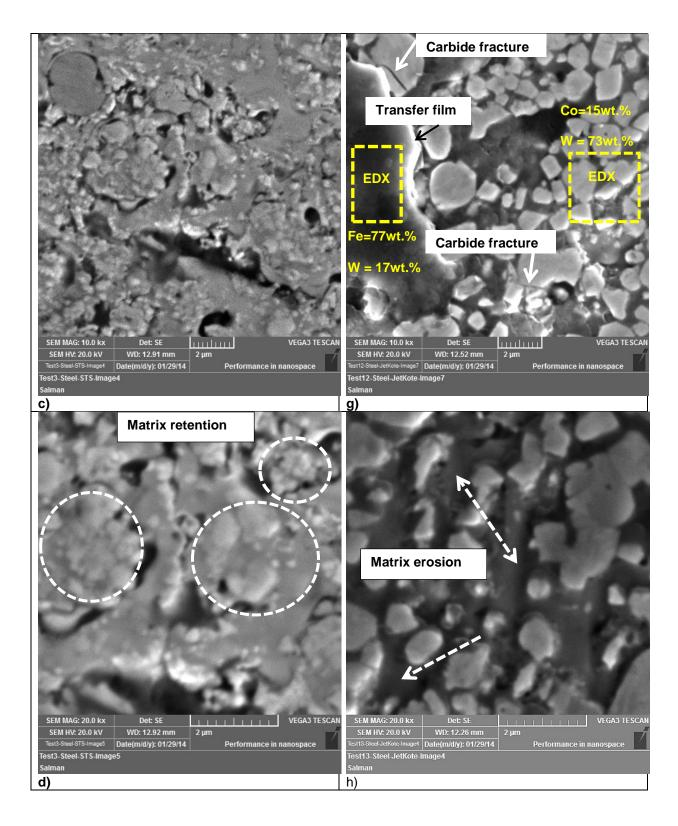
**Figure 18**, SEM Observations of the wear tracks of coatings deposited under spray conditions; a,b,c,d) # 2 and e,f,g,h) # 3. EDX analysis at two different location marked by boxes is shown in caption (g).
