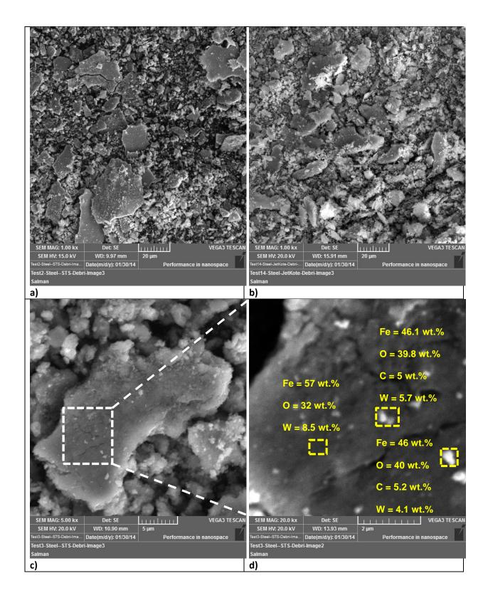
**Figure 19**, SEM Observations of the wear debris resulting from wear tests for test couples deposited under spray conditions a) #2 and b) #3, c) high magnification image of debris for spray condition # 2 indicating the location of EDX analysis, d) EDX analysis at three different locations marked with boxes.
