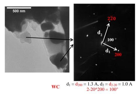
Figure 7: Experimental diffraction pattern (DP) from a particle coated under deposition condition # 1. The DP matches with WC.
