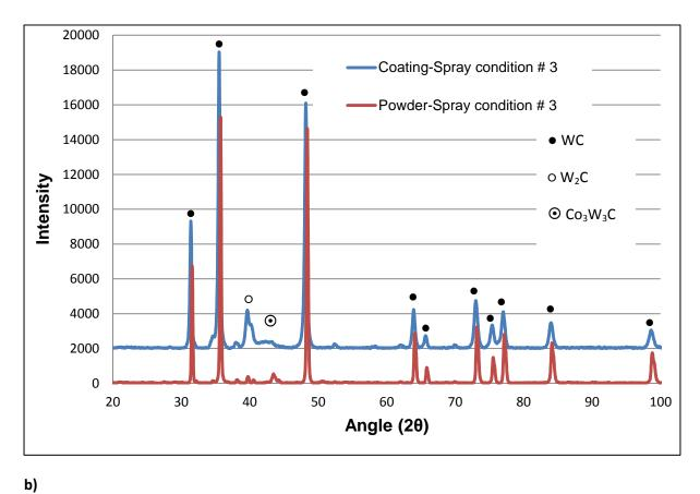
Figure 4, XRD pattern of spray powder and coating for deposition conditions # a) 1, 2 and b) 3.
