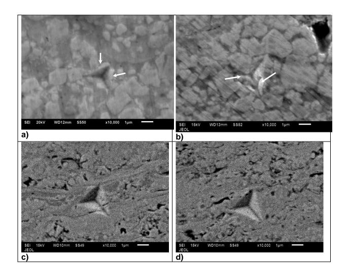
**Figure 15**, SEM observations of nanoindents at 50mN load for a,b) conventional HVOF coatings (deposition condition # 3), c,d) S-HVOF coatings (deposition condition # 2). Arrows marked in caption a) indicate material pile-up, whereas in caption b) indicate carbide fracture.
