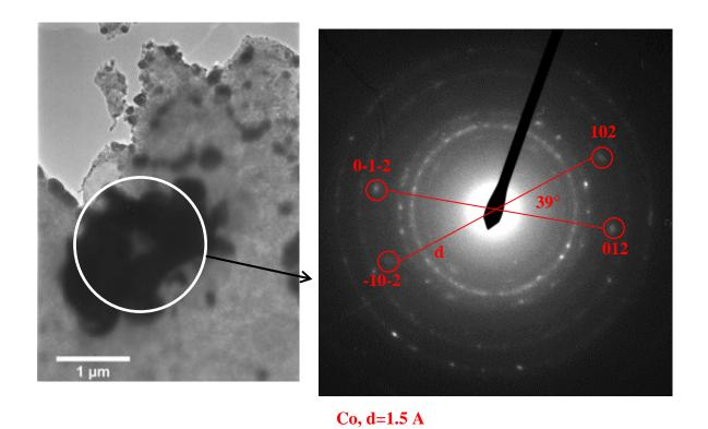
Figure 9: Observation of diffraction pattern from a thick region of the sample coated under deposition condition # 1: apparition of new diffraction spots probably linked to Co.
