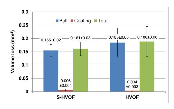
**Figure 16**, Volume loss results for the ball-on-plate sliding wear tests for S-HVOF (Deposition condition # 2) and HVOF (Deposition condition # 3) coatings.
