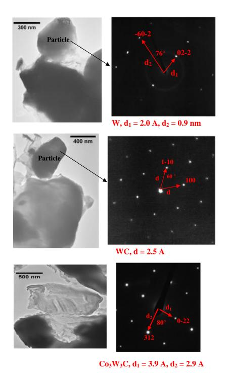
Figure 10: Observation of single crystal oxide particles with different orientations for coated sample under deposition condition # 2. They are identified as W, WC and  $Co_3W_3C$ .
