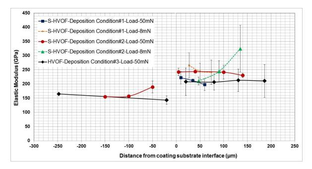
**Figure 14**, Reduced elastic modulus results of coating substrate systems deposited under deposition conditions # 1, 2, 3. Zero at x-axis represents the location of coating-substrate interface and the distances represented are measured from this interface.
