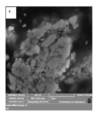
**Figure 1**, SEM observations of the a) agglomerated and sintered WC-12 wt.% Co spray powder, b) nano-structured powder after milling, c) cross-section of milled powder.
