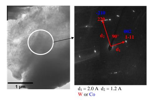
Figure 11: Near single crystalline diffraction pattern from the thick region of the sample coated under deposition condition # 2. The DP may be linked to W and/or Co.
