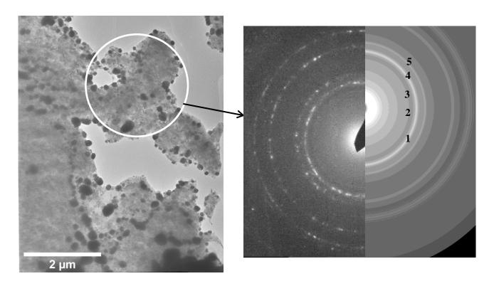
Figure 8: Diffraction pattern of coated sample under deposition condition # 1 plane view sample.
