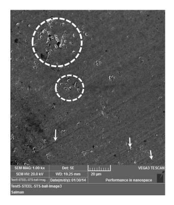
**Figure 20**, SEM Observations of the worn steel ball surface. The white arrows indicate the location of abrasive marks, whereas the dotted circle indicates the location of surface pits due to plastic deformation.
