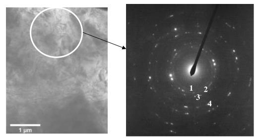
Figure 12: Diffraction pattern from a thin region of the sample coated under deposition condition # 2.
